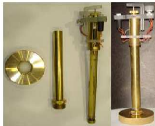
Diagram.1 Transient Hotwire Thermal Conductivity Measuring Apparatus
